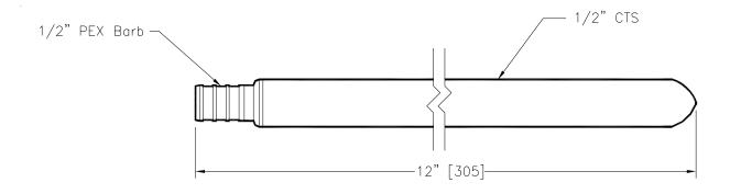
**Engineering Specification:** ZurnPEX<sup>®</sup> 1/2" Straight Copper StubOut. 1/2" PEX Barb x 1/2" CTS. End spun closed allows for system testing before valves or other fittings are installed. Meets NSF® and ASTM requirements.
