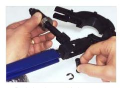
Push the pin out with the screw driver until you can grab it with your fingers, then remove the pin and screw/nut assembly from the tool.
