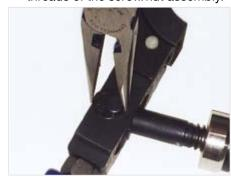
('We recommend an extreme pressure lubricant such as white Lubriplate or the lubricant sold for the screw drives of Genie garage door openers.) To apply lubricant, turn the nut counter clockwise by hand until it stops at the end of the screw. Apply a small amount of lubricant to the threads at the midway point of the screw. Spin the nut up and down the screw a few times by hand to distribute the lubricant. Wipe off any excess lubricant with a rag.
