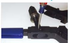
If necessary, remove existing E-Clip by prying it away from the pin with a flat head screw driver.
