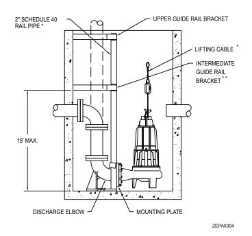
Guide rail system is for removal and installation of flanged, horizontal discharge pumps without getting in or removing fluid from pit.
