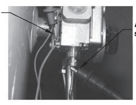
Alligator clip to copper sheath of thermocouple
