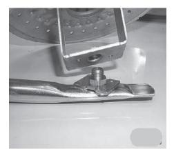
Step 5. Remove main burner orifice from feed line. Inspect and clean if necessary.
