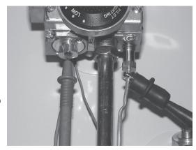
Step 3. If continuity is indicated, the ECO is O.K.. If continuity is not indicated, the ECO has opened, and the gas valve must be replaced.
